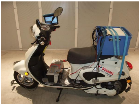
Figure 4 E-Scooter (left) and C-Scooter (right) with attached near-field microphones and mobile data acquisition device (multi-channel front-end in the blue box)
