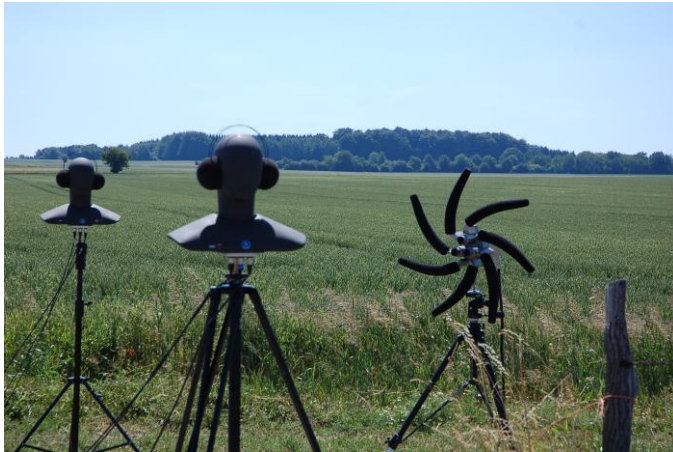
Figure 3 Left: Picture of the stationary measurement set-up with artificial head and visor microphone array Right: Fully equipped C-Scooter during pass-by measurement
