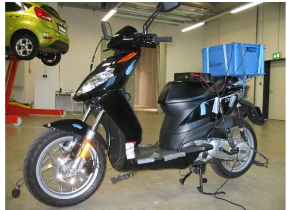
Figure 4 E-Scooter (left) and C-Scooter (right) with attached near-field microphones and mobile data acquisition device (multi-channel front-end in the blue box)
