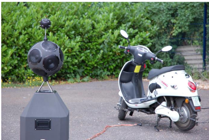
Figure 12 Measurement set-up to determine the source related transfer functions (SRTF).
