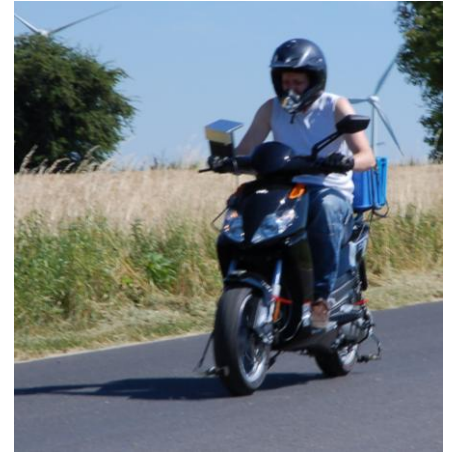
Figure 3 Left: Picture of the stationary measurement set-up with artificial head and visor microphone array Right: Fully equipped C-Scooter during pass-by measurement
