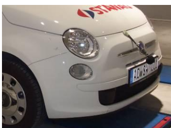
Microphone in front of engine compartment
