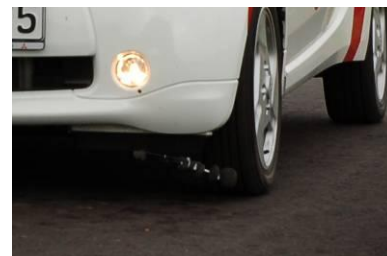
Microphone front left tyre inlet
