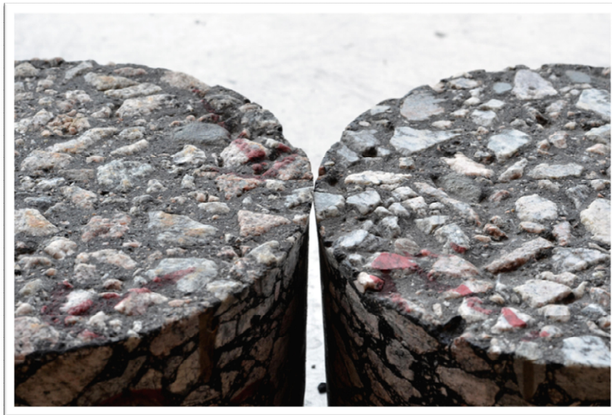
Figure 2.4 Comparison between a not grinded and a grinded sample.
