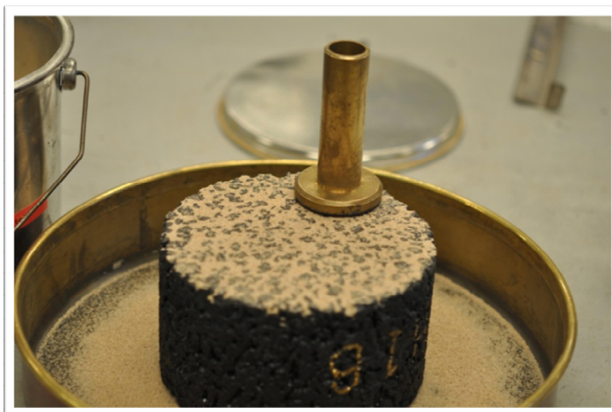
Figure 2.2 Measuring sand-patch value on a core.
