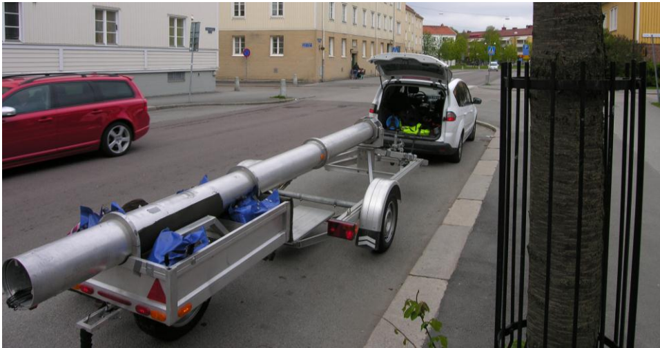
Figure 3. Single wheel trailer for CPX-measurements
