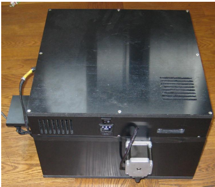
Figure 1. Laser scanner developed for road texture measurements.
