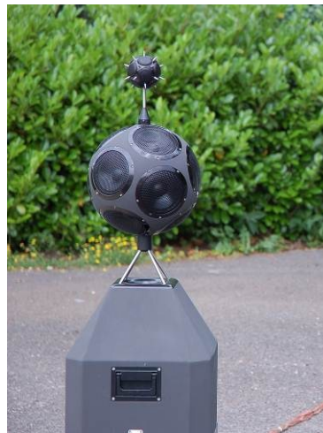
Figure 13: Dodecahedron measurement system for the determination of source related transfer functions (SRTF).
