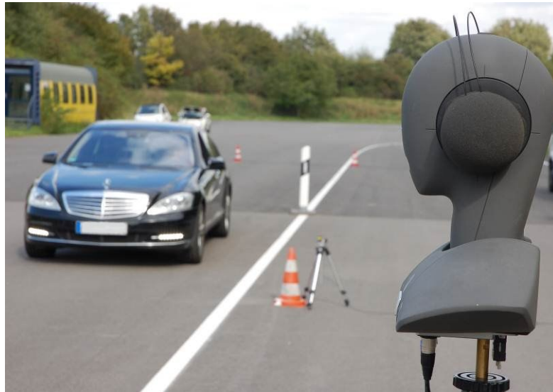
Figure 14: Artificial head system measuring single pass-by noise events on a test track
