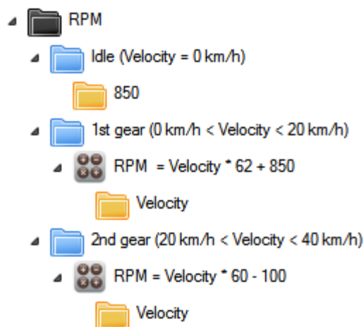
Figure 4: Example for a driving condition model. The information of the vehicle velocity is used to calculate the engine speed.
