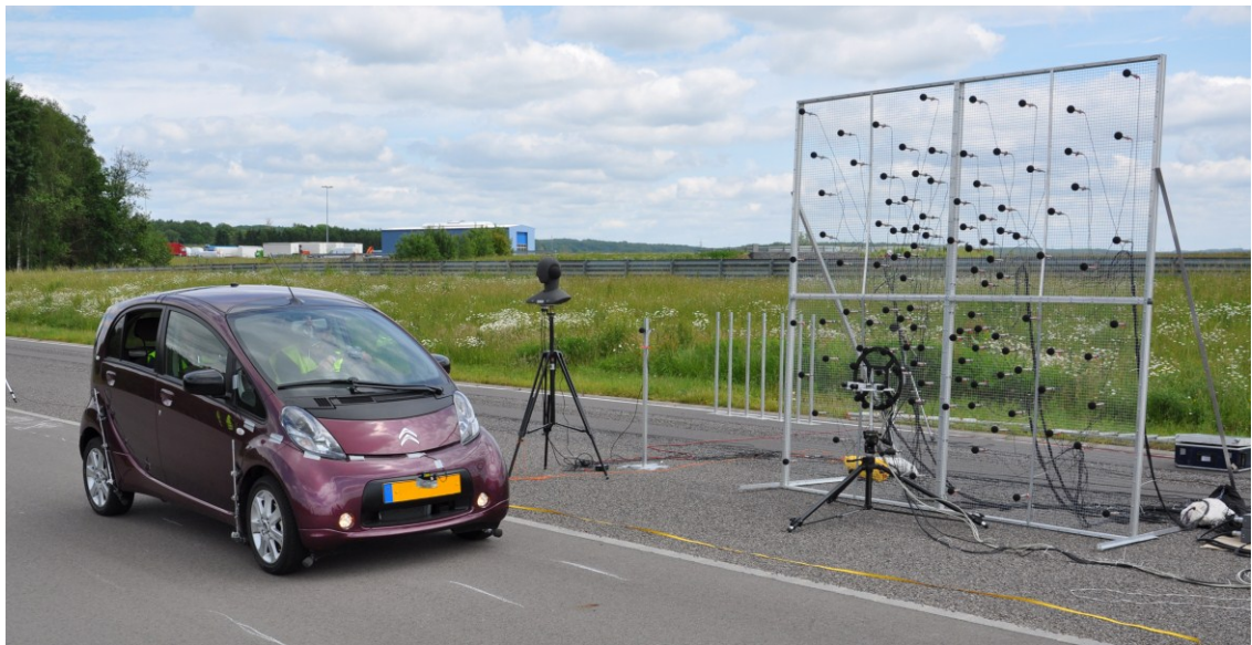
Figure 30: Stationary measurement setup for measuring Citroën C-Zero
