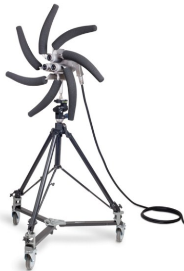
Figure 15: Standard beamforming array optimized for application in industrial application (left), flexible large scale array for measurement of road traffic
