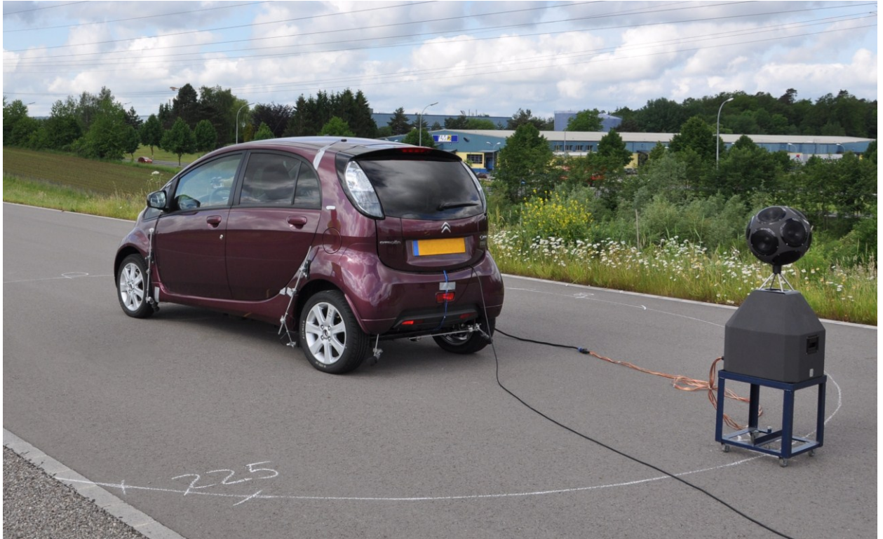
Figure 42: Measurement setup for SRTF measurements with dodecahedron
