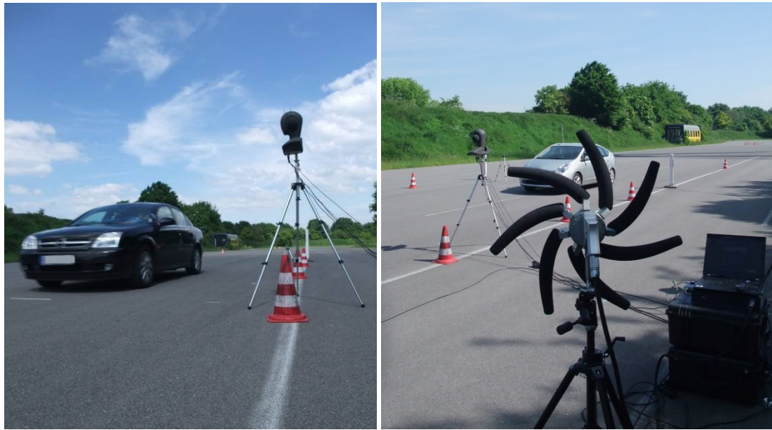
Figure 21: Pass-by measurement of an Opel Vectra (combustion engine, left) and a Toyota Prius (hybrid drive, right) on a test track
