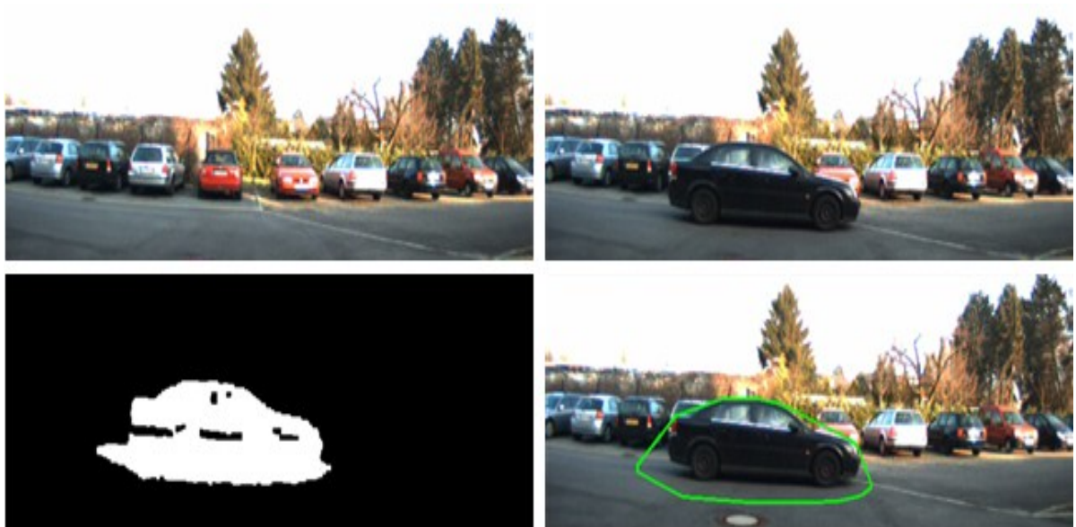
Figure 17: Detection of moving vehicles: background image (upper left image). Moving object (upper right image), foreground detection (lower left image) and contour detection (lower right image)
